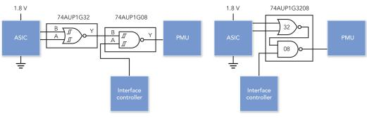
Configuration A: Discrete logic solution
